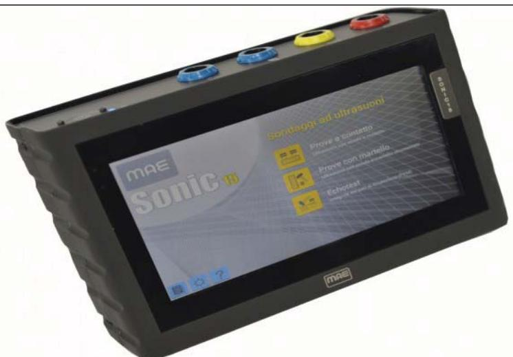
SONIC15 is a device for non Destructive Tests and surveys which uses ultrasonic pulse velocity and sonic tests on masonry with instrumented hammer. It supports extension, too for surveys on foundation piles with P.I.T. methodology. In spite of compact dimension of the unit, there is a wide monitor of 7" with integrated touch screen which allows to use it in immediate and effective way during construction.
