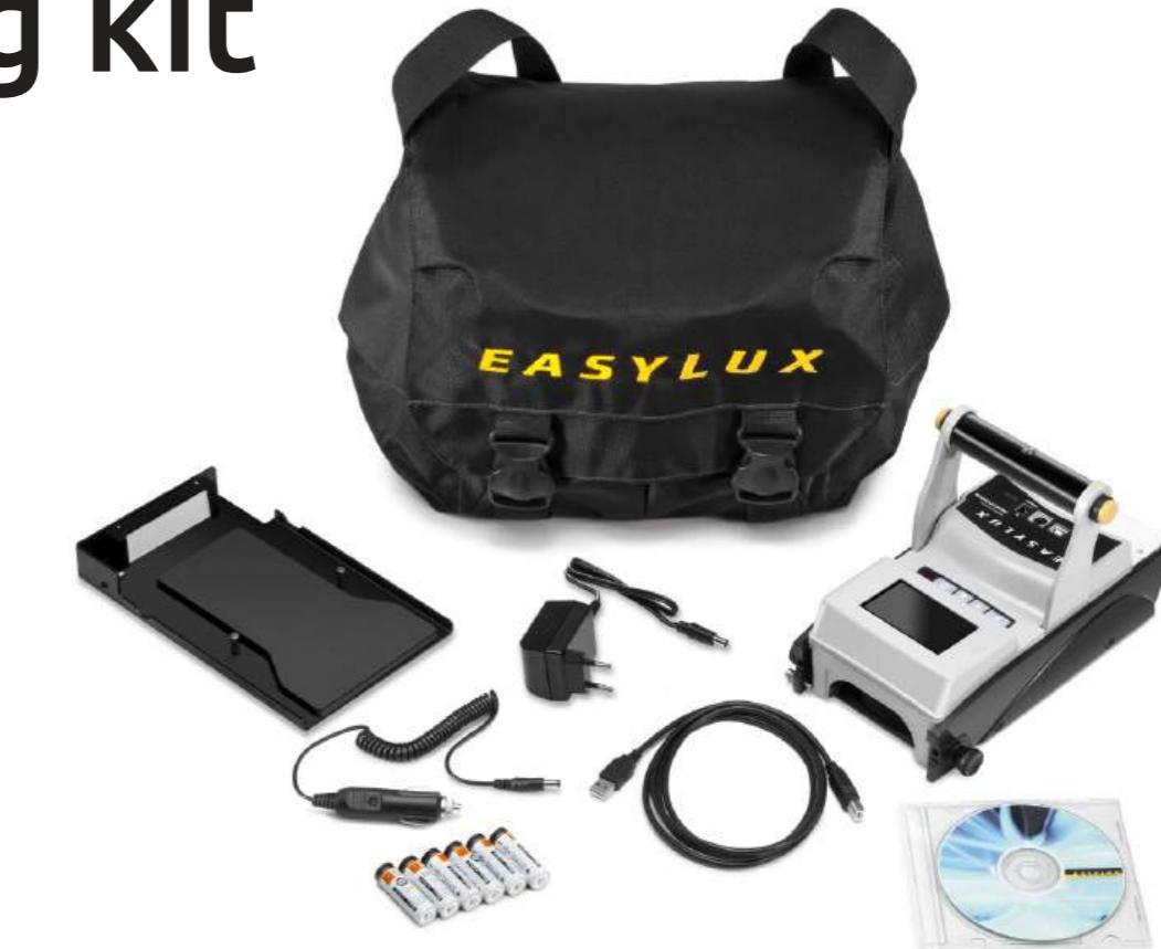
MiniReflecto Horizontal measures the night visibility **RL**, the Day Visibility **Qd**, the visibility under wet **RL** **wet** and continuous wetting conditions **RL-2 rain** of all shapes and colors of road markings, even **RL** profiled up to 15 mm without adjustments.
