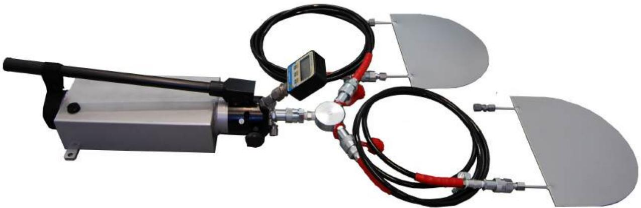
The flat jack method is a diagnostic test used for buildings and masonry.
